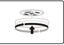
**④Rotate the lamp clockwise** and install onto base plate, then finish installation!
