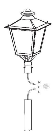
Step 3. Wire the cable with the cable in the pole.
