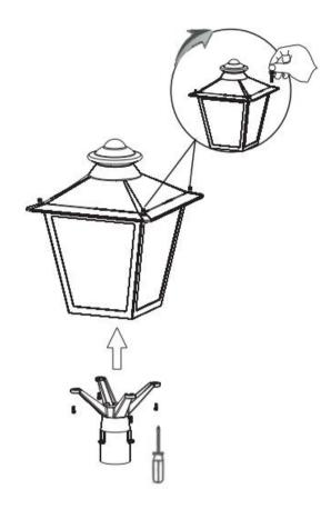
Step 2.Close the top cover of the fixture, and fix the top cover onto the fixture using screws. And then after use screw driver to fix the mount bracket to the fixture.
