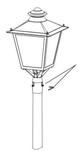
Step 4. Use screws to fix the fixture onto the pole.
