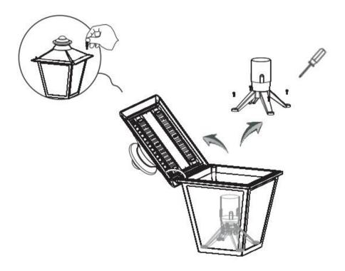
Step 1.Use your hand or tools to loosen the 2 screws on the top of the fixture, open the top cover of the fixture, and then take out the mount bracket inside the fixture.
